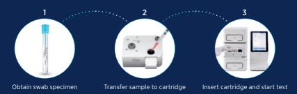
**Just add your sample.** Idylla<sup>™</sup> will take care of the rest. Our fully automated test enables detection of SARS-CoV-2 virus in about 90 minutes – from sample input to result reporting.
